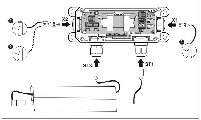
● Slack-rope switch ● Pass-door switch
