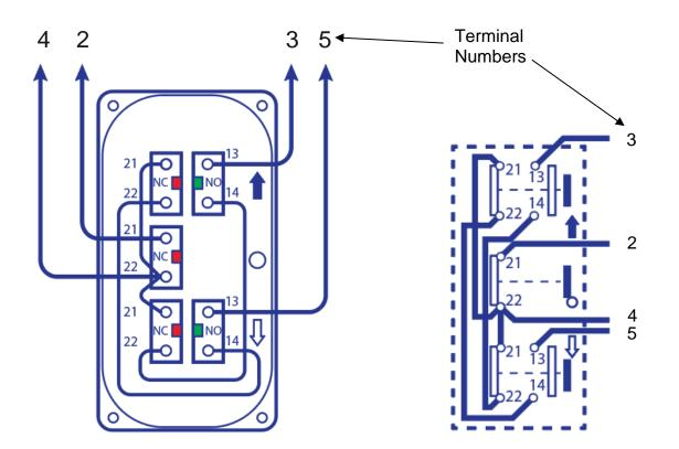
Direct wiring of a 24Vdc alarm signal (normally energised, de-energised in alarm) without FCP03
