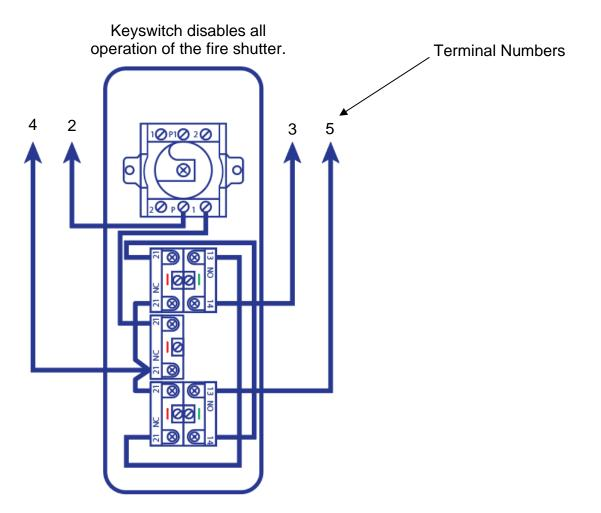
N.B. For Hold-to-run (deadman) operation do not connect to terminal number 4
