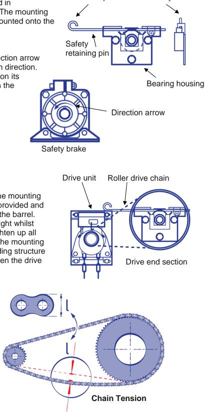
Ensure pin seated correctly
