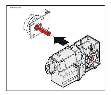
► Tighten all connection elements (M8) to 25 Nm. Install all other connection elements according to the specifications of the door manufacturer.
