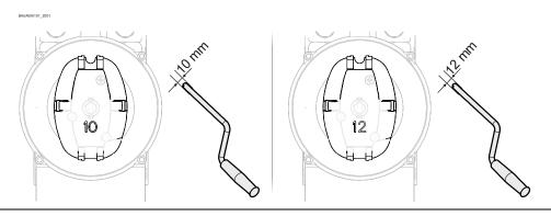
Plug in the crank and turn until it engages (1). Open or close by turning the crank (2).
