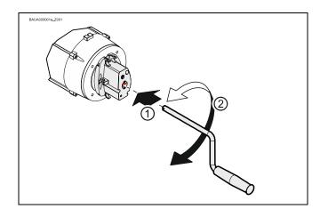
After use, the crank may be attached to the drive unit.
