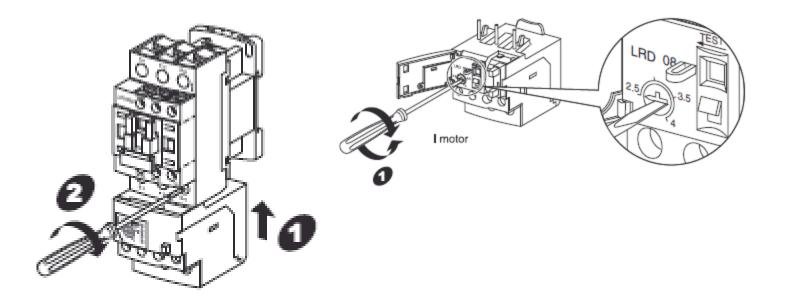
Adjust the overload to suit the motor current rating.
