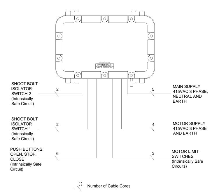
Intrinsically Safe Circuits must be run separately from other non-intrinsically safe circuits. Cables of intrinsically safe circuits must be protected from mechanical damage, identified light blue and enter the enclosure through light blue cable glands.
