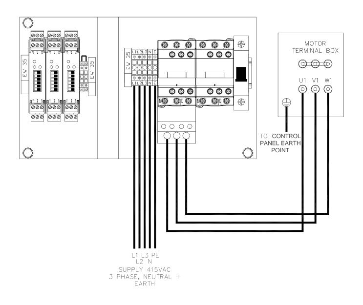
All cables must enter the enclosures through the pre-drilled and tapped holes using correctly fitted EExd rated cable glands.
