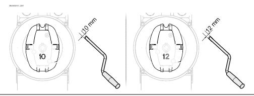
Plug in the crank and turn until it engages (①). Open or close by turning the crank (②).
