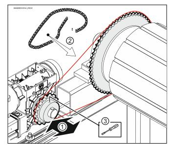
Tighten the chain wheel properly (①/②). Tighten all connection elements (M12) to 75 Nm (③). Install all other connection elements according to the specifications of the door manufacturer.
