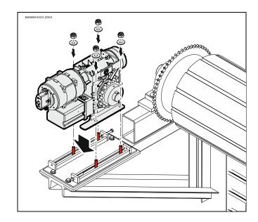
Position the chain wheel (1) properly. Install the chain wheel (2). Secure the chain wheel (3).
