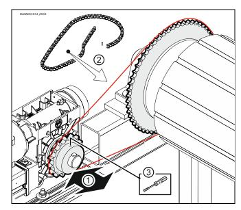
Tighten the chain wheel properly (①/②).
