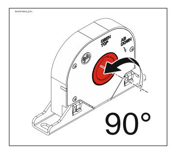
Press the red plunger back into the housing.
