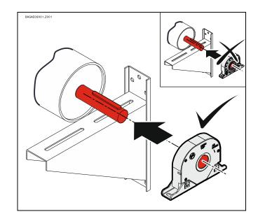
Tighten all connection elements (M12) with a torque of 75 Nm. Install all further connection elements according to the specifications of the door or facility manufacturer.
