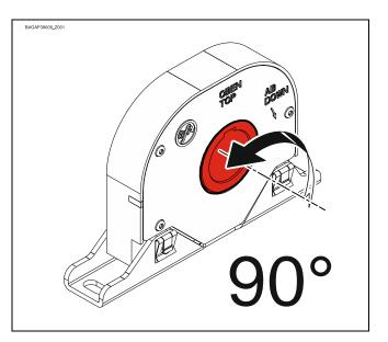
Press the red plunger back into the housing. The safety brake is ready for operation again.
