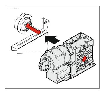
Tighten all connection elements (M12) to 75 Nm. Install all other connection elements according to the specifications of the door manufacturer.
