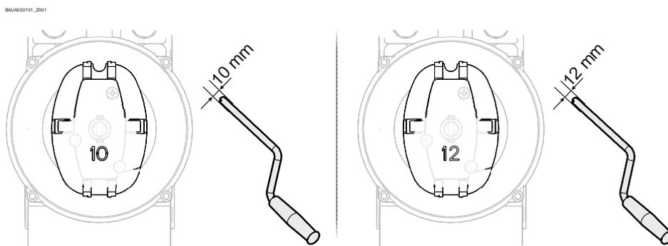
Plug in the crank and turn until it engages (①). Open or close by turning the crank (②).
