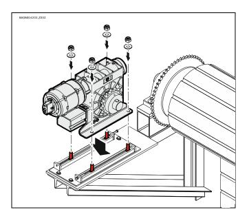
Position the chain wheel (①) properly. Install the chain wheel (②). Secure the chain wheel (③).
