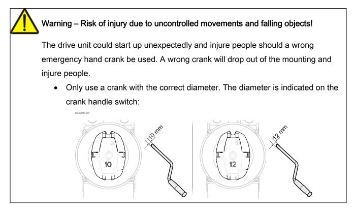
Plug in the crank and turn until it engages (①). Open or close by turning the crank (②).
