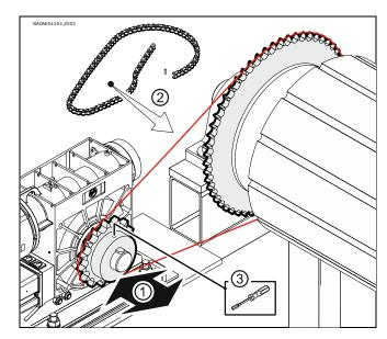
Tighten the chain wheel properly (①/②).
