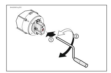
After use, the crank may be attached to the drive unit.
