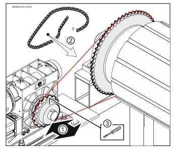
Tighten the chain wheel properly (①/②). Tighten all connection elements (M16) to 175 Nm (③). Install all other connection elements according to the specifications of the door manufacturer.
