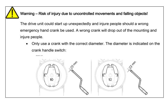
Plug in the crank and turn until it engages (①). Open or close by turning the crank (②).
