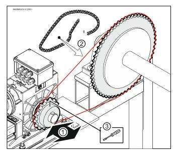
Correctly tension the chain (①/②). Tighten all connection elements (M12) with 75 Nm (③). Install all further connection elements according to the specifications of the door manufacturer.
