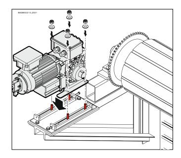
Correctly position the sprocket (①). Mount the chain (②). Fixate the sprocket (③).
