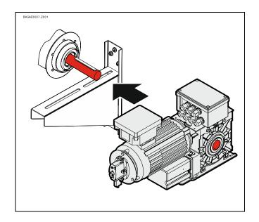
Tighten all connection elements (M12) with a torque of 75 Nm. Install all further connection elements according to the specifications of the door manufacturer.
