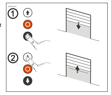
The OPEN final limit position can be corrected by following the fine adjustment procedure. Check the door position after each correction.
