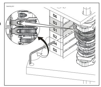
The S1 EMERGENCY OPEN limit switch is preset by the setting of the OPEN final limit position. The door must stop without posing any risks should the rotating direction be incorrect or should there be a fault with the S3 OPEN limit switch. Follow the fine adjustment procedure to correct the switching point of the limit switch as needed.
