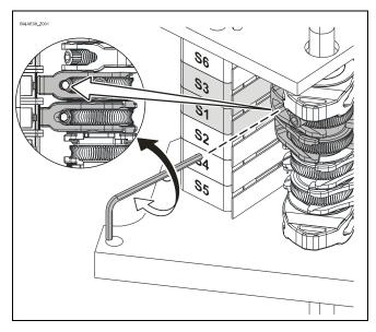
The S1 EMERGENCY OPEN limit switch is preset by the setting of the OPEN final limit position. The door must stop without posing any risks should the rotating direction be incorrect or should there be a fault with the S3 OPEN limit switch. Follow the fine adjustment procedure to correct the switching point of the limit switch as needed.
