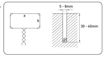
Recommended loop wire: H05 V-K, 0.75 mm<sup>2</sup>. At a cross-section of 1.5 mm<sup>2</sup>, the loop feed may be up to 100 m long. The loop feed must be well-twisted (min. 20 times / m) and should not be laid parallel to power lines.
